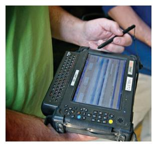
in barcode reader-runs on Windows and operates the same bisTrack software as all the other computers within the company. It even shows the standard screens that the counter salesmen see. The device is made to handle the wear and tear of life in the lumberyard, as well as do its job even in cold New England winter mornings.
