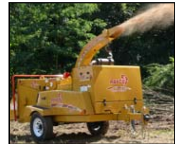
12-inch Capacity Drum-Style Brush Chipper
