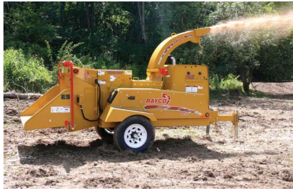
12-inch Capacity Drum-Style Brush Chipper
